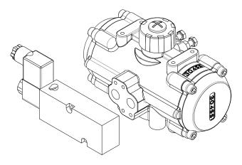
MOUNT SOLENOID IN POSITION SHOWN. USE THE TWO MOUNTING HOLES NOTED TO ALIGN O-RINGS AND SOLENOID TO THE ACTUATOR
