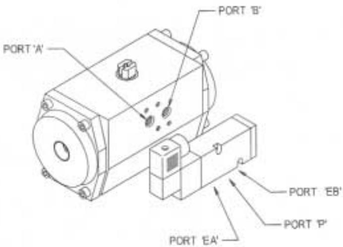
**MOUNT SOLENOID IN POSITION SHOWN. USE THE TWO MOUNTING HOLES NOTED TO ALIGN O-RINGS AND SOLENOID TO THE ACTUATOR**
